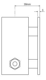
Note: The Assembly is shown with 1/4@ OD tube fittings. The dimensions across the tube fittings will vary for all other size fittings.
